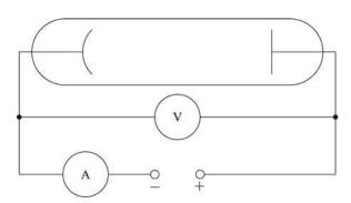
power supply negative connected to detector; ammeter and voltmeter correctly connected; *Allow voltmeter connected directly across power supply.*
